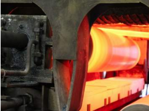
Descaling operations in process at a Rolling Mill.
