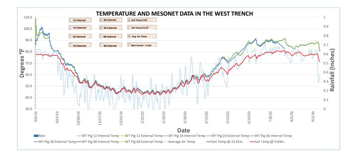
Figure 70. Ambient air, ambient soil, and trench temperatures in the west trench
