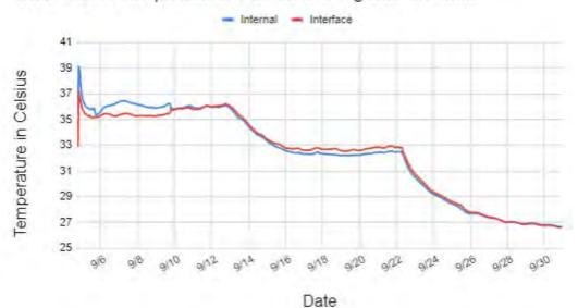
West Trench Temperatures Internal and Pig/Soil Interface
