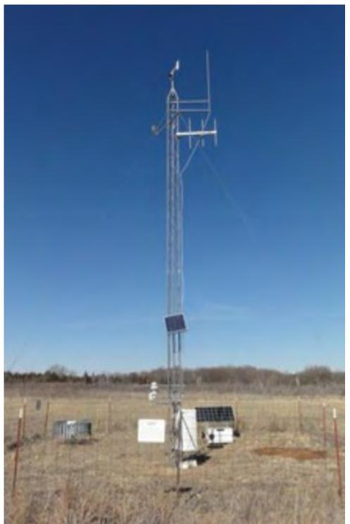
environmental measuring instruments located on or near a 10-meter-tall tower. The measurements are packaged into "observations," then transmitted to a central facility 24 hours per day year-round. The
