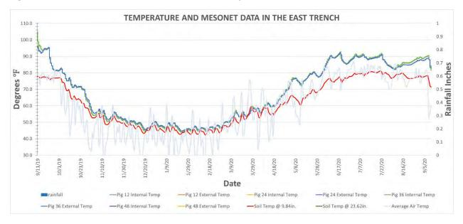
Figure 70. Ambient air, ambient soil, and trench temperatures in the east trench
