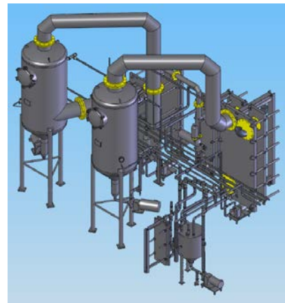
SIGMASTAR®-45 Evaporator Plant
