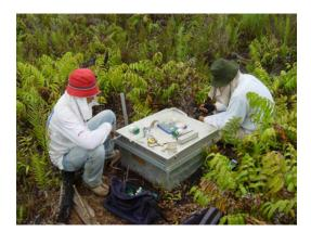
Figure 7.5: GHG flux measurements. a) Gas sampling for greenhouse gas flux determination by the closed chamber method in clear felled burned peatland at Ex-Megarice area, Central Kalimantan. Photo: Jyrki Jauhiainen.
