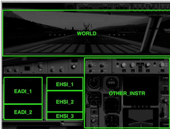
Figure 4. Definition of the AOIs on the cockpit of the Boeing 737-900ER.
