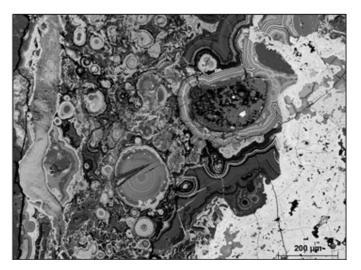
Figure 4. Colloidal cements at Taron.
