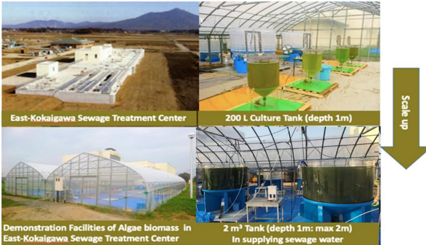
Figure 7: Algae biomass production system in Kokaigawa East Sewage Treatment Center. (University of Tsukuba et al, 2020).
