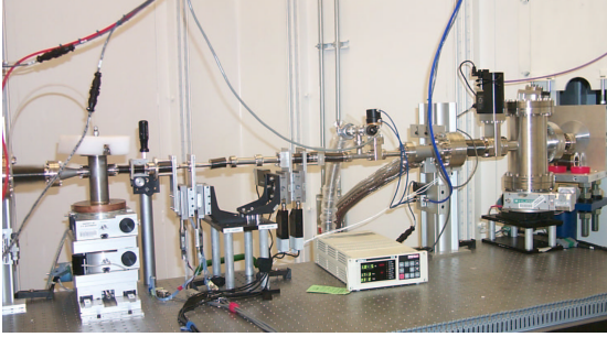
FIG. 3: Picture of the 8-ID XPCS setup. Key components from right to left are: monochromator, beam-cross-section-defining slits, guard slits, sample chamber. The CCD is not shown and is located 3 m further to the left.
