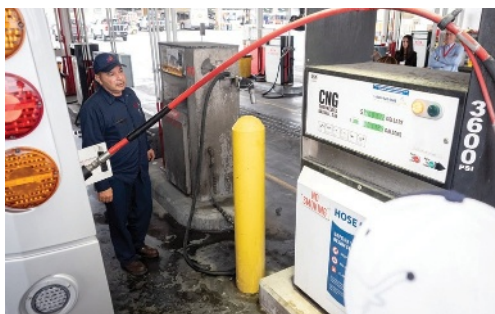
A CNG bus undergoes fueling at VIA Metropolitan Transit's fueling station.
