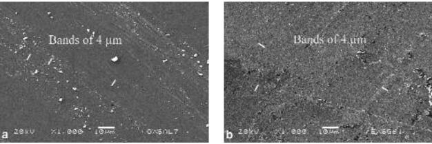
Figure 7. Archaeological polishing (a) and experimental polishing with chert (b) at 1000x.
