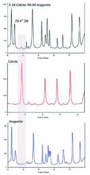
**Figure 1.** XRD spectra of (a) mixture of 0.1% calcite in 99.9% aragonite; (b) pure geological calcite; and (c) pure biogenic aragonite. Despite the broad peak overlap, the (114) peak at 29.4°  $2\Theta$  angle (range indicated by shadowing) is characteristic of calcite and is evident in binary mixtures of as low as 0.1% calcite.
