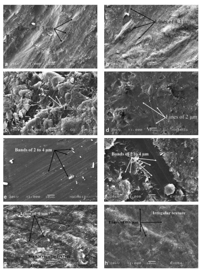
Figure 7. SEM comparisons between experimentally drilled holes and archaeological ones: (a and b) using sand and reed; (c and d) using obsidian flakes; (e and f) using chert burins; (g) using powder of chert, (h) and using volcanic ash with reed.
