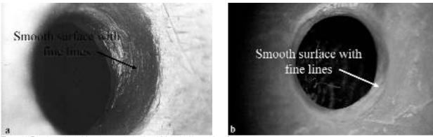
Figure 11. Experimental hole (a) and archaeological bead (b), both with smooth surface.
