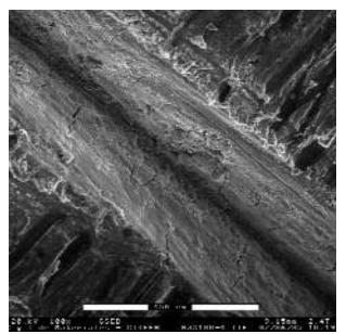
Figure 4. Lithic cut-mark left in bone (B3). Close V-shaped profile. ESEM. 100X.
