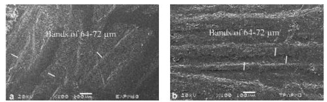
Figure 8. Experimental abrading with andesite (a) and archaeological one (b), both at 100X.
