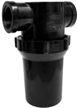
Strainer 3/4" NPT 200 Mesh (80 Micron) Strainer recommended on all MixRite installations
