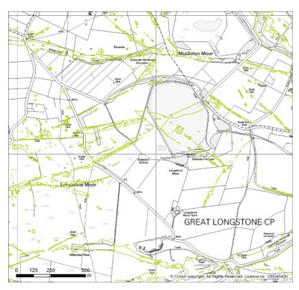
Figure 4.1.3 Extract of aerial photograph transcription showing the network of lead rakes and associated lead mining remains on and around Longstone Moor. The settling lagoon in the centre of the illustration also shows the impact that modern industry can have on landscape-scale remains
