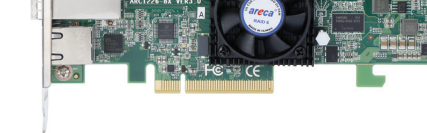
ARC-1226-8x 2 x SFF-8644 8 x 12Gb/s SAS ports up to 8 drives
