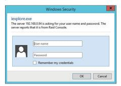
Type the User Name and Password. The RAID controller default User Name is "admin" and the Password is "0000". After entering the user name and password, click the button to access the storage manager.
