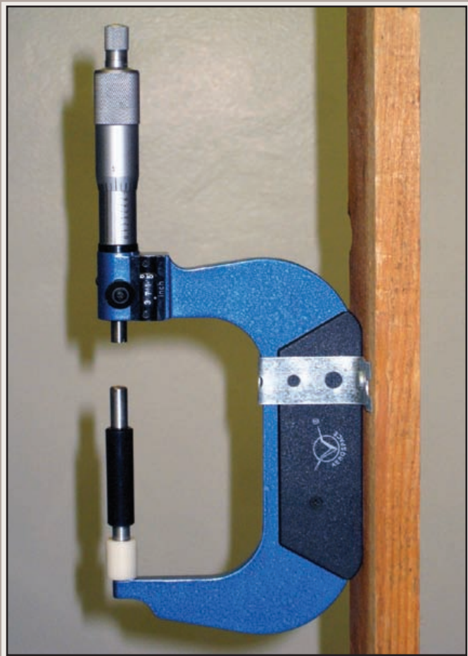
FIG. 1. Micrometer (4-inch), fitted with the 3-inch insert and machined white plastic collar to hold the insert in place, and shown attached to the wooden stand that was used for support in the field. This configuration allowed measurement of shell heights of up to 25 mm (one inch). Shell heights between 25–100 mm (1–4 in) could be measured by using either of the two shorter inserts (for 25–50 mm or 50–75 mm shells) or no insert (75–100 mm shells).
