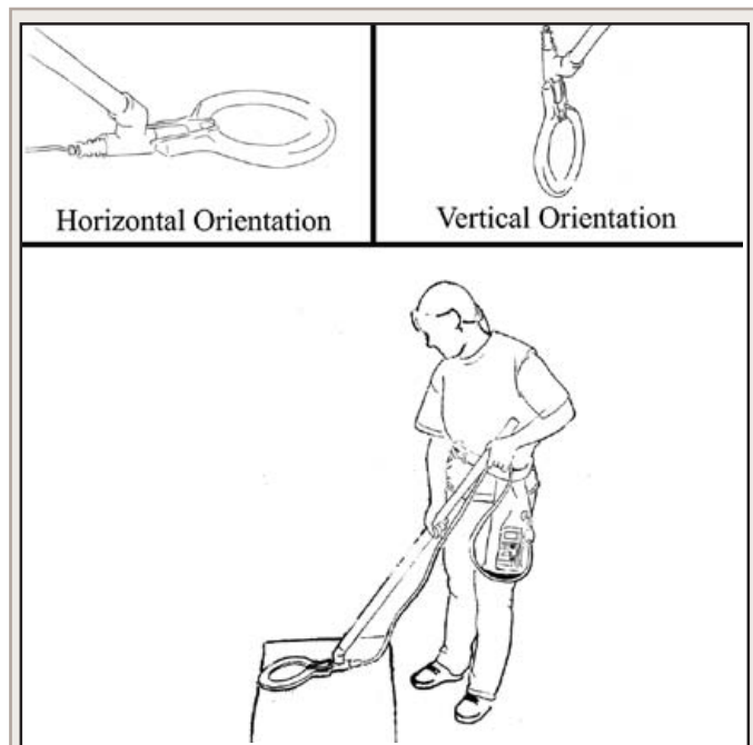
FIG. 1 Horizontal and vertical orientation of the antenna hoop and illustration of how to scan a coverboard with PIT-tag reader.
