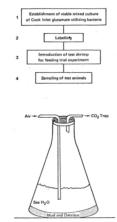
Appendix Figure 3. Experimental set up for closed mini-ecosystem approach. The test chamber is a specially modified 6 L Ehrlenmeyer flask.
