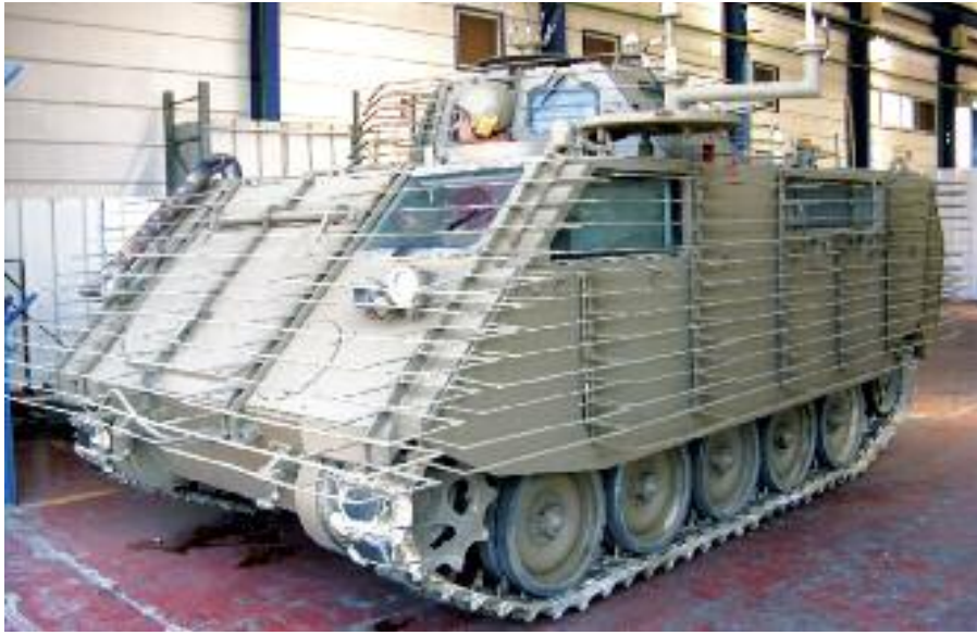
An M113 armoured personnel carrier equipped with Israel Military Industries Iron Wall passive anti-RPG system – a mix of passive and bar armour. (IMI)
