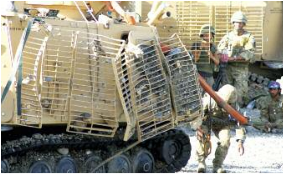
A damaged cage armour fixed onto a Danish BV206. Cage armour are a statistic protection system, the average probability being around 60%. (Danish MoD)
