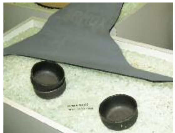
SSAB is currently working on ways of making its armour steel solutions more formable. Here is an example of Armox 500 formability. (Armada – P. Valpolini)
