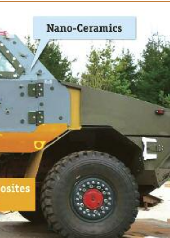
Iveco’s MPV exploits the latest IBD Deisenroth armour developments, mostly based on nanotechnologies. (IBD)
