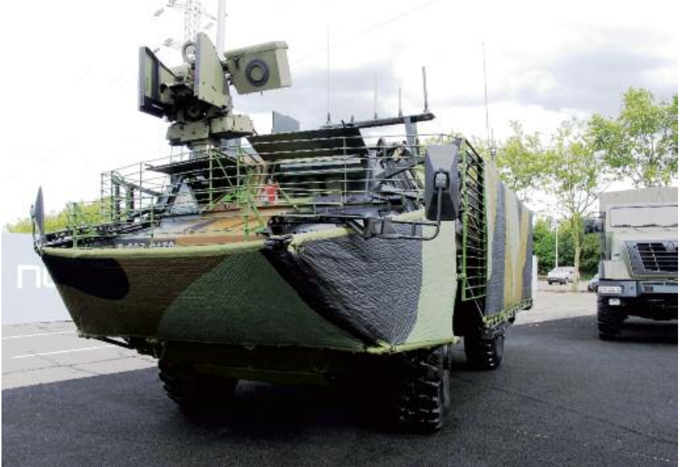
A Renault Trucks Defense VAB Mk3 exhibited at Eurosatory 2012 modelled the various elements of the Ultra Flex Family, an RPG protection system developed by Plasan Sasa. (Armada/P. Valpolini)
