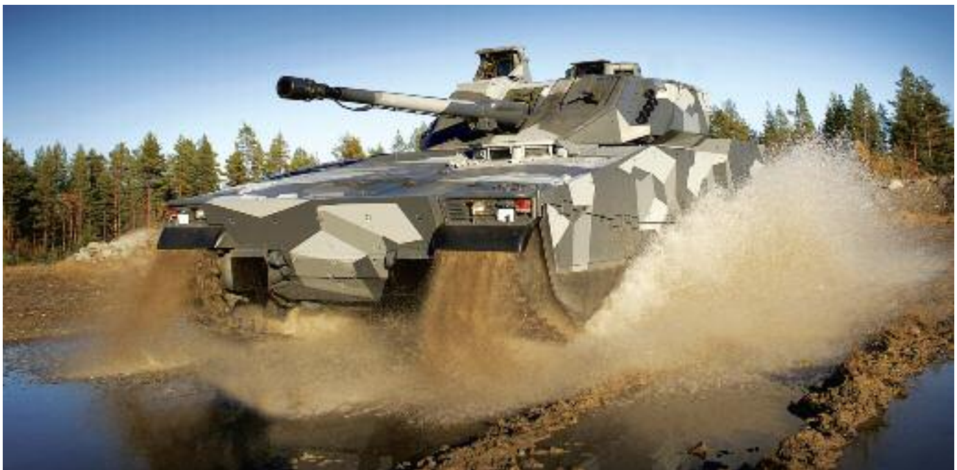
A CV90 prototype equipped with Saab Leds sensors. The protection device's hard-kill effector is the Saab Avitronics Moongoose 1 missile. (Saab)
