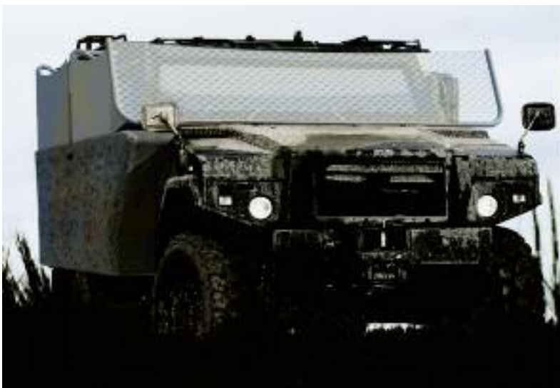
Montage shows the Falanx solution installed over a Mowag Eagle with both the net and opaque options used to provide full protection of the vehicle, while the graphical representation of the system over a Piranha depicts its effectiveness. (Falanx)
