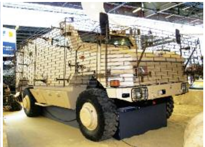
Nexter has developed its own RPG bar armour system known as PG Guard, here mounted on the company's VBCI (left), and Aravis (right). Its effectiveness is rated at 50 to 65 per cent depending on the type of RPG warhead countered. (Armada – P. Valpolini)
