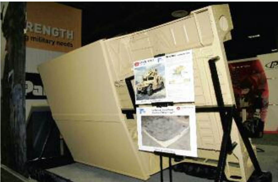
Ceradyne and Cellular Materials International developed an underbelly protection system based on CMI MicroTruss, an aluminium cellular material that allows to absorb about one third of the energy generated by the explosion. (Armada/P. Valpolini)
