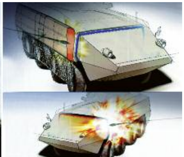
Montage shows the Falanx solution installed over a Mowag Eagle with both the net and opaque options used to provide full protection of the vehicle, while the graphical representation of the system over a Piranha depicts its effectiveness. (Falanx)
