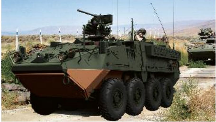
Ruag further developed its SidePro KE/IED, here seen in a photo montage, to counter those new devices that generate multiple fragments. (Ruag)
