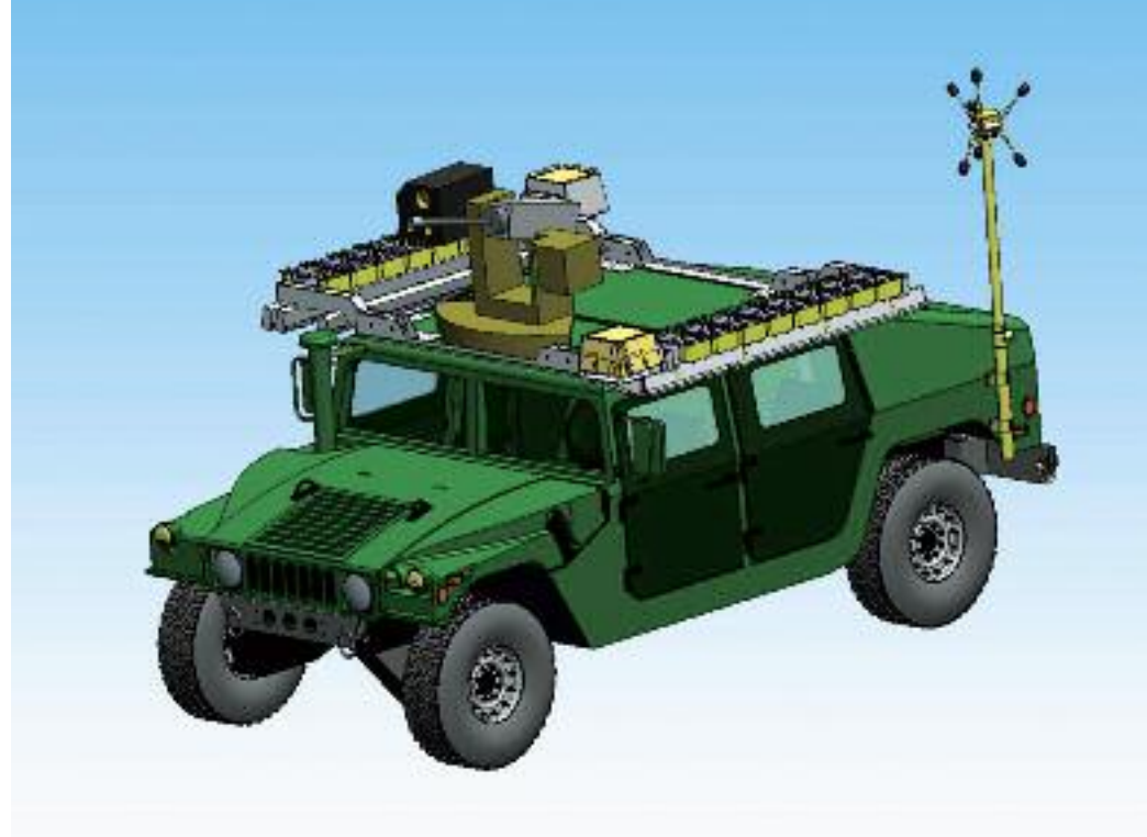
A pictorial of the Crosshair – Iron Curtain system that puts together an active defence system and an acoustic location system, developed under the auspices of the Darpa. According to some information the system has been tested in Afghanistan. (Darpa)
