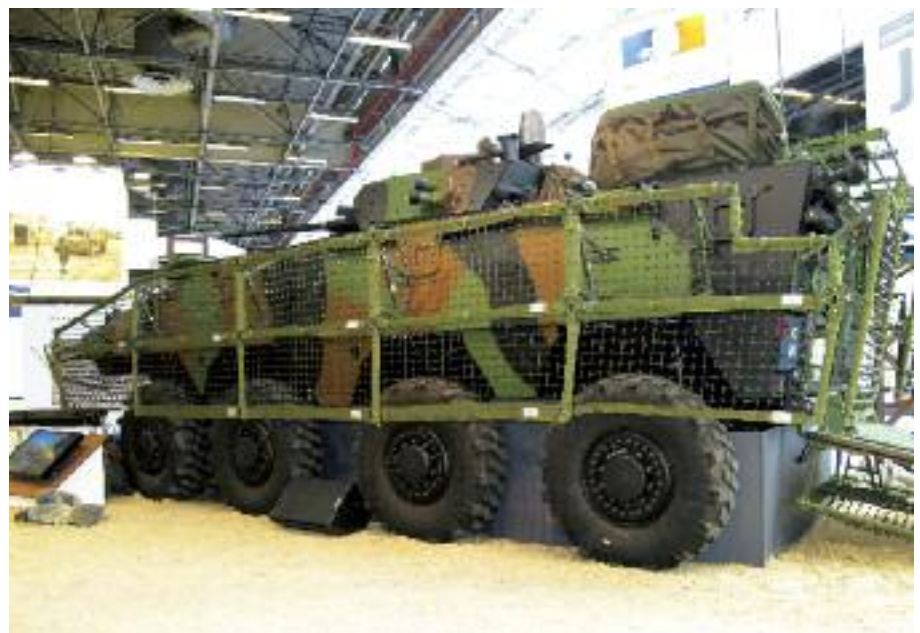
French Army VBCI operating in Afghanistan are equipped with QinetiQ North America Q-Net, a net system with embedded metal nodes. (Armada/P. Valpolini)
