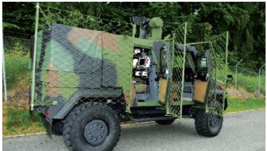
The Ruag SidePro Lasso, here mounted on an Eagle, is designed to preserve maximum accessibility to the vehicle. It has been adopted by Denmark, Slovenia and Estonia. (Ruag)
