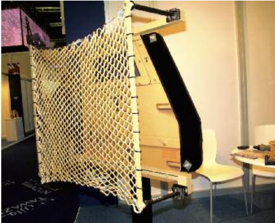
A close up of the Tarian, the net anti-RPG system produced by AmSafe in Britain, exhibited at IDEX; the stand-off distance is of about 250 mm, which is typical of those systems. The actual net was made of a fake fabric to avoid industrial intelligence. (Armada/P. Valpolini)
