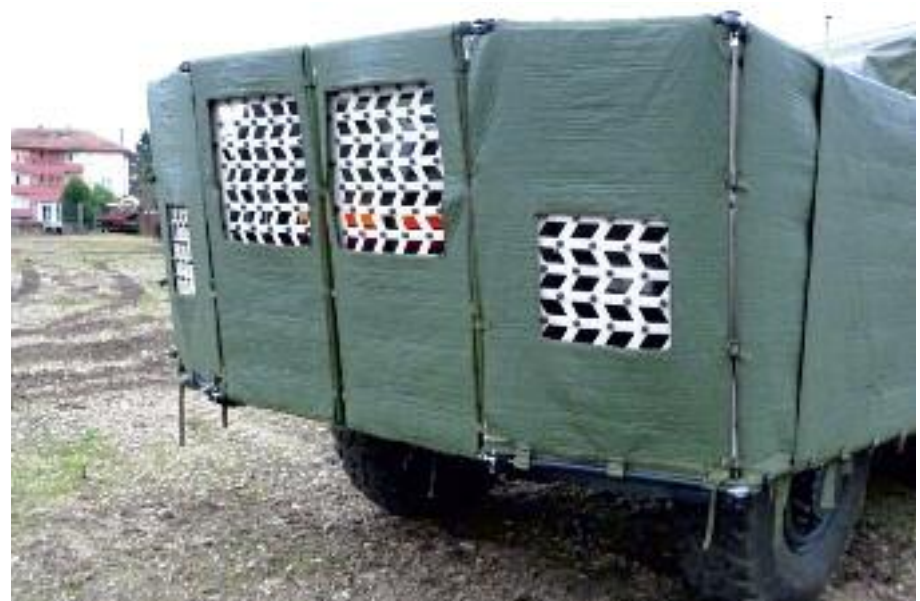
The back of the VAB Mk3 shows the Light Fence's transparent elements that are being used in front of windows with the exception of the windscreen. (Plasan Sasa)
