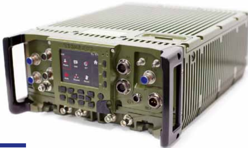
Thales' vehicular CONTACT transceiver is displayed here. The firm's CONTACT radio family will be interoperable with the PR4G radios in French military services which the new radios will replace.
