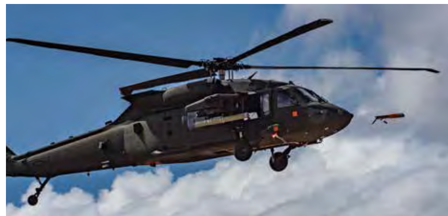
Air Launched Effects Demonstration: Area-I ALTIUS (Agile-Launch, Tactically Integrated, Unmanned System) horizontal launch from a UH-60.
