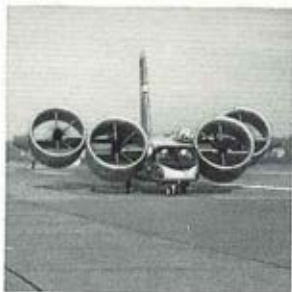
For takeoff, the four ducted propellers are rotated to the vertical thrust position. At the desired altitude, they are transitioned gradually to the horizontal thrust position for forward flight. The sequence is reversed for vertical landing.
