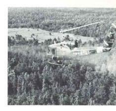
Daylight gunnery begins with the four 7.62-mm machine guns, two on each side of the UH-1.
