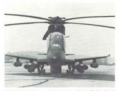
STRATFORD, CONN. — Sikorsky Aircraft's S-67 Blackhawk demonstrates its firepower capability by carrying 152 2.75inch anti-personnel rockets. They are designated FFAR for Folding Fin Aircraft Rockets. The turret beneath the fuselage can carry either 20mm or 30mm cannon. The Blackhawk, the world's fastest helicopter, can also be equipped with other missiles and rockets to make it a highly lethal anti-tank weapons system. Among this armament is the TOW missile system.
