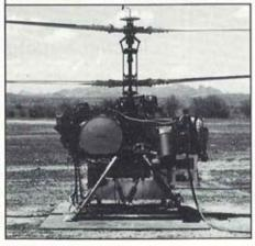
QH-50 Helicopter Drone Target used for Airto-Air Stinger testing. Research and Development:
