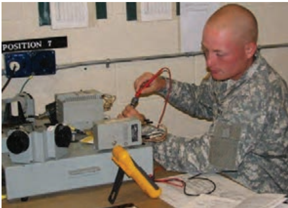
A 15N student following troubleshooting procedures on Radar Warning System Trainer.
