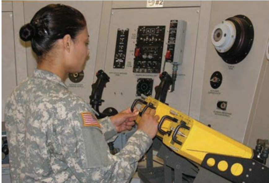
A 15N student performing Maintenance Operational Check on CMWS trainer.
