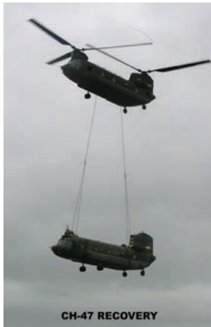
CH-47 using a Unit Maintenance Aerial Recovery Kit (UMARK) during a CH-47 and UH-60 recovery.
