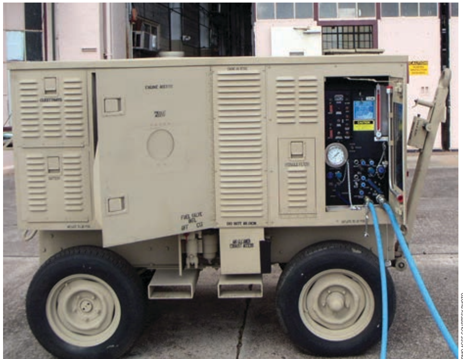
Aviation Ground Power Unit.
