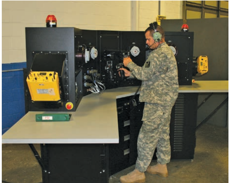
The Common Missile Warning System Maintenance Trainer-Apache (CMT-A) – The CMT-A replicates the CMT with the addition of simulated aircraft system compartments to give the maintainer the difficulty of performing maintenance tasks as if on the actual aircraft.
