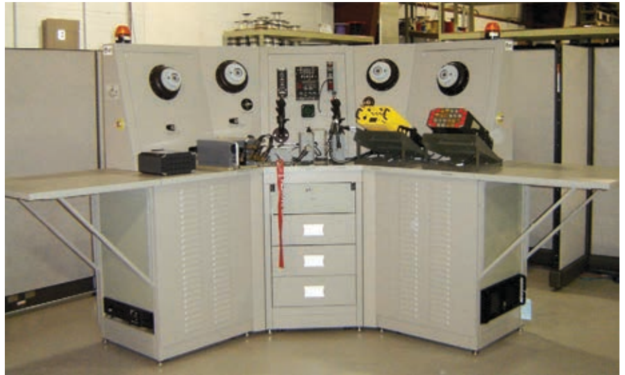
A Common Missile Warning System Maintenance Trainer (CMT) – The device supports operations, fault isolation, and line replacement unit (LRU) maintenance training tasks. The CMT configuration replicates the CH-47 in a bench type environment.
