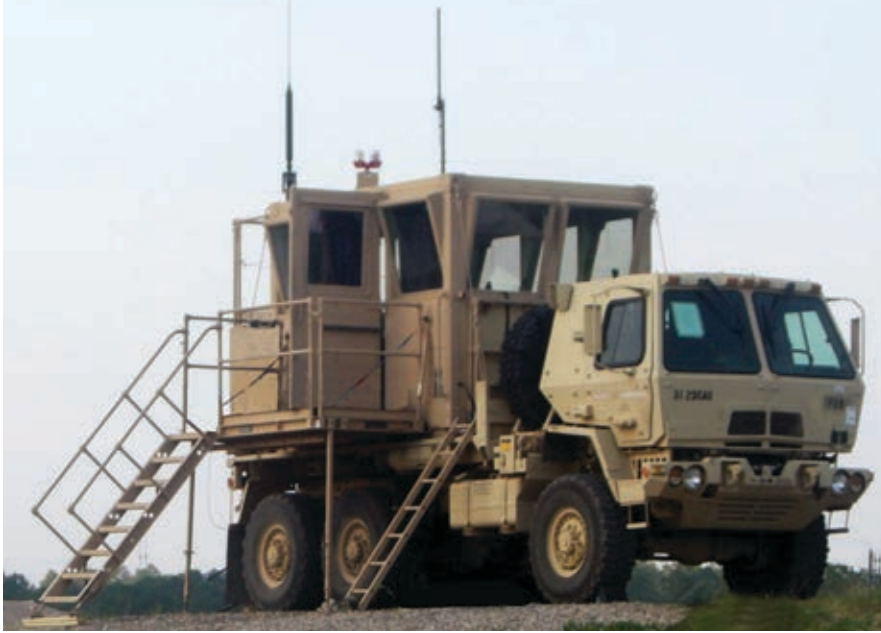
The Mobile Tower System (MOTS) is a rapidly deployable air traffic control tower that supports operations at military/civilian airfields and tactical landing zones worldwide.
