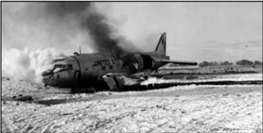
Figure 12.2. Crash landing of a Marine aircraft flown by Capt. (USMC) Paul Noel and two crew members. The crash occurred after the plane's load of ammunition shifted when the aircraft touched down on a hard-scrabble airstrip. Remarkably, all three crew members survived the crash. Courtesy of the National Archive and Records Administration.
