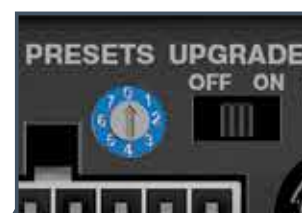
AP bit amplifiers have 7 Drive preset for 7 different system configuration selectable by a switch in the front panel without PC software.
