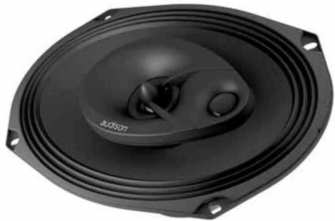
The 40 mm horn loading dome tweeter contributing to maximize efficiency to increase it up to 96 dB SPL. The acoustics lens is specifically designed and applied to the tweeter to increase dispersion in high frequency range.
