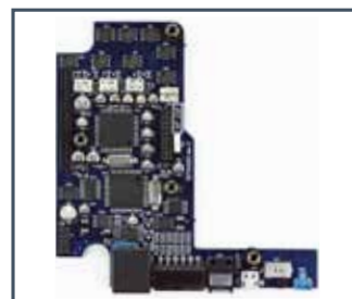
The AP bit amplifiers built-in processor provides the ability to set new performance standards for OEM Integration, ensuring full compatibility with the bit Drive technology. Through the management software, the powerful 32 bit DSP ensures all the functionalities which made the Audison bit One and bit Ten renowned worldwide.
