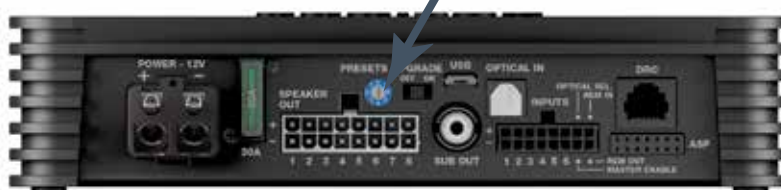
AP bit amplifiers have 7 Drive preset for 7 different system configuration selectable by a switch in the front panel without PC software.
