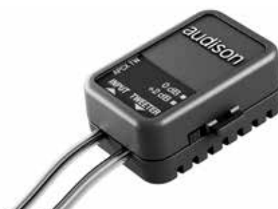
The AP 1 tweeter is provided with an extremely small sized dedicated passive crossover featuring an attenuation switch (0 dB, +2 dB) to correct the response in the car compartment according to the different installation conditions.
