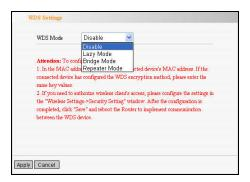
**Lazy:** In this mode, the connected device can be Bridge mode or Repeater mode and enter the Router's BSSID
