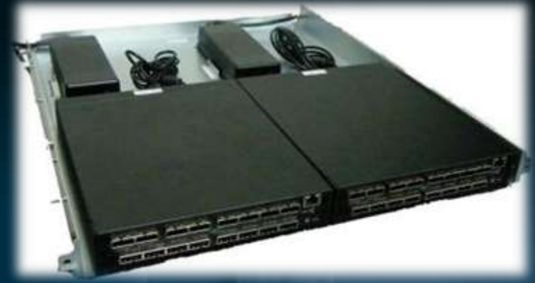
Two SAS6160 Switches in a 19" Rack
