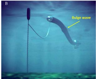
Figure 5.6. Examples of A) a submerged pressure device: © CWE 2011. A CETO™ device. B) an example of a completely different device design: © Checkmate Sea Energy 2012. Artist's impression of an Anaconda™ device.
