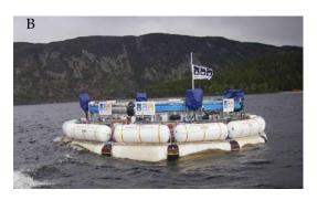
Figure 5.2. Examples of point absorbers: A) © Wave Star A/S 2011. The Wave Star™ 1:2 scale demonstration plant in Hanstholm, DK; B) © AWS Ocean Energy 2010. A 1:9 scale model of the AWS-III™ device being tested in Loch Ness, Scotland, UK; C) © OPT 2012. A PowerBuoy™ device.
