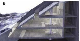
Figure 5.5. Examples of overtopping devices: A)  $\odot$  WaveDragon 2011. A WaveDragon<sup>TM</sup> device. B)  $\odot$  SSG 2005. Artists' impression of the Seawave Slot-Cone Generator<sup>TM</sup>.
