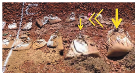
Figure 6. Damaged sample bags
