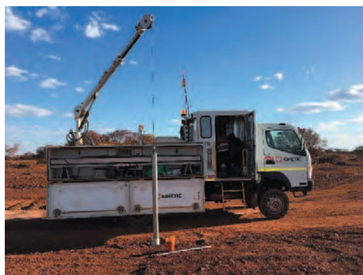
Figure 1. The FastGrade™ being run in hole
