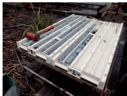
Figure 6. TCGA01 drill core (serpentinite). Image courtesy of Joe Xie and Yunnan Tin.
