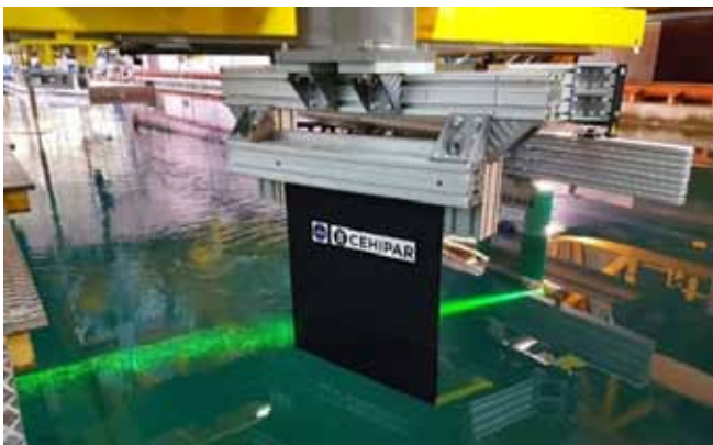
PIV system in action in the calm water tank
