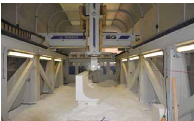
CNC machine milling a mould
