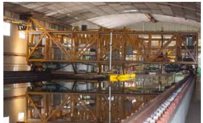
Towing test experiment in the calm water tank
