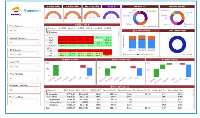
Figure 3. Repsol Control Tower dashboard including capacity utilization, customer service and demand fulfillment, monomer balances, and detailed economics such as netbacks, costs and prices.
