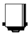
BA 15s DIN: 49720 IEC: 7004-11A ANSI: Single contact candelabra bayonet base C81.61-1990 sheet I-20-1
