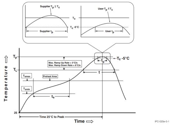
Figure 5-3: Reflow Profile from IPC/JEDEC J-STD-020E (Not to Scale)
