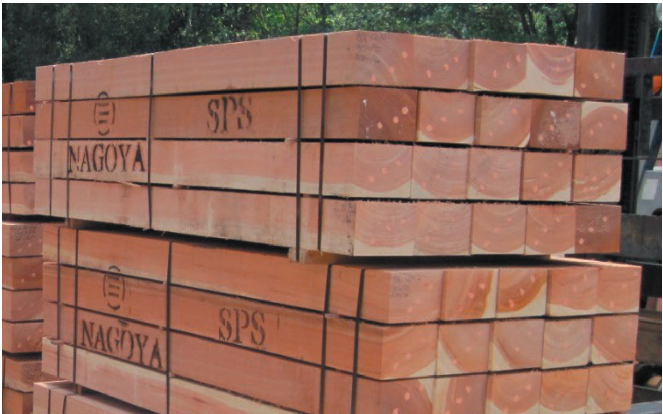
Crossings made of Kempas (photo: Benoit Gomet, France Timber, Nagoya, Japan)
