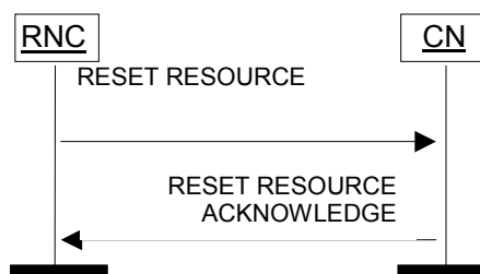
Figure 34: RNC initiated Reset Resource procedure. Successful operation.
