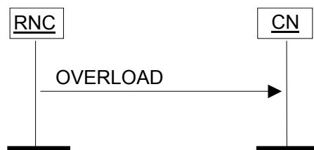
Figure 28: Overload at the UTRAN. Successful operation.
