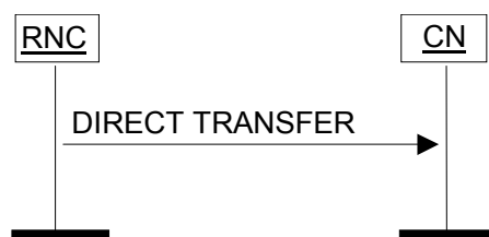
Figure 26: Direct Transfer, RNC originated. Successful operation.
