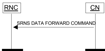
Figure 13: SRNS Data Forwarding Initiation procedure. Successful operation.
