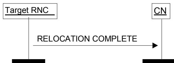
Figure 10: Relocation Complete procedure. Successful operation.
