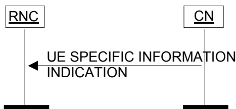
Figure 40A: UE Specific Information procedure. Successful operation.
