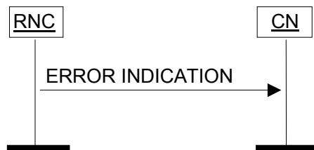
Figure 32: Error Indication procedure, RNC originated. Successful operation.
