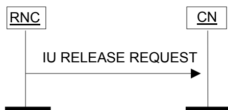
Figure 3: Iu Release Request procedure. Successful operation.
