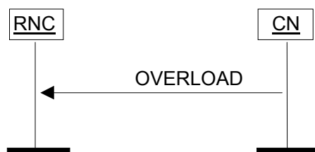
Figure 27: Overload at the CN. Successful operation.
