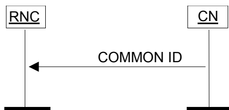
Figure 17: Common ID procedure. Successful operation.
