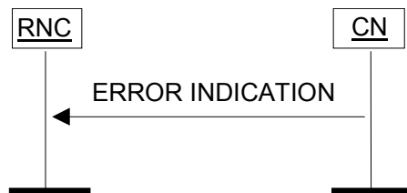
Figure 31: Error Indication procedure, CN originated. Successful operation.
