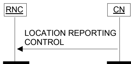
Figure 21: Location Reporting Control procedure. Successful operation.
