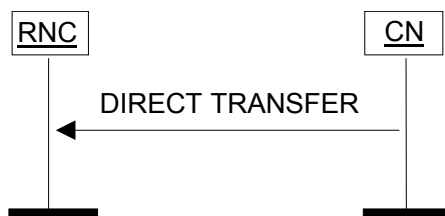
Figure 25: Direct Transfer, CN originated. Successful operation.
