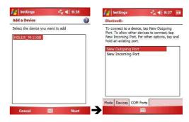
8. Select the COM port, then tap finish, it will show as right figure, and tap "OK" to finish the Bluetooth setting. Recommend not to use "Secure Connection" which may cause unstable connection.
