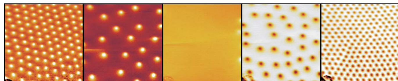
Figure 3: MFM measurements at different magnetic fields: Left to right: B = -40 Oe, -10 Oe, 0 Oe, +10 Oe, +50 Oe. Scan size is 10 \times 10 \mu\text{m}^2 , color span is 2 Hz for all images.
