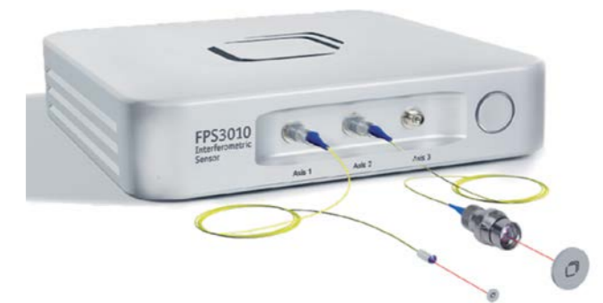
Figure 2: attocube's 3-axes real time interferometer, the FPS3010, features 25\ \text{pm} resolution and a measurement bandwidth of 10\ \text{MHz} . The fiber based measurement heads are available in sizes from 4 to 14\ \text{mm} diameter dependent on the application. These heads are also compatible with ultra-high vacuum as well as cryogenic conditions.
