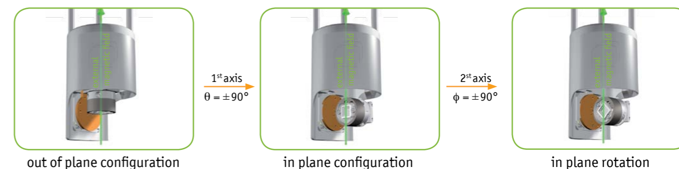
Figure 1: Working principle. The first rotation axis controls the orientation of the sample plane with respect to the fixed external magnetic field ( \theta: \pm 90^\circ ), whereas the second rotator actuates the in-plane component ( \phi: \pm 90^\circ ). Combining both axes allows for arbitrary mutual orientations of the magnetic field vector with regards to the sample plane.
