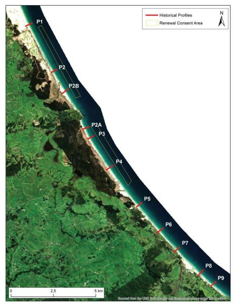
Figure 2.1: Location of historical beach profiles used in shoreline position/volume and bathymetry change monitoring under existing MBL extraction consents
