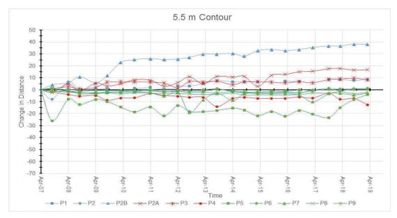
Figure 4.2: Excursion Distance plot of the 5.5m contour (proxy of dune face position) at historic profile sites 2007 – 2019.
