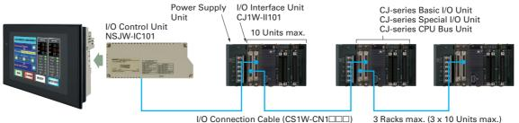
Note: Maximum of 3 Racks for models with model numbers with a suffix of -G5D, and 1 Rack for models with model numbers with a suffix of -M3D.
