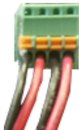
Figure 5-20: Wires Inserted in Terminal Block
