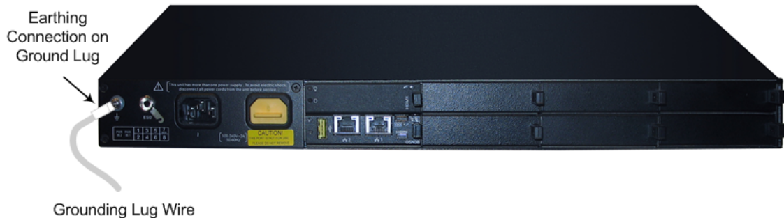
Figure 5-1: Grounding the Device
