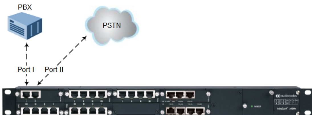
Figure 5-17: Cabling (Ports 1 and 2) PSTN Fallback
