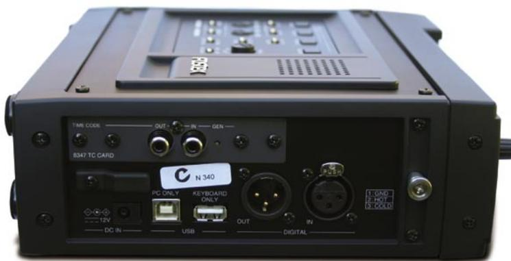
terminate in a four-pin XLR. Fostex has fitted only a domestic DC input, which doesn't offer you the security of a latching professional connector. That said, my 2.1AH lead-acid will run the Fostex for well over four hours.
