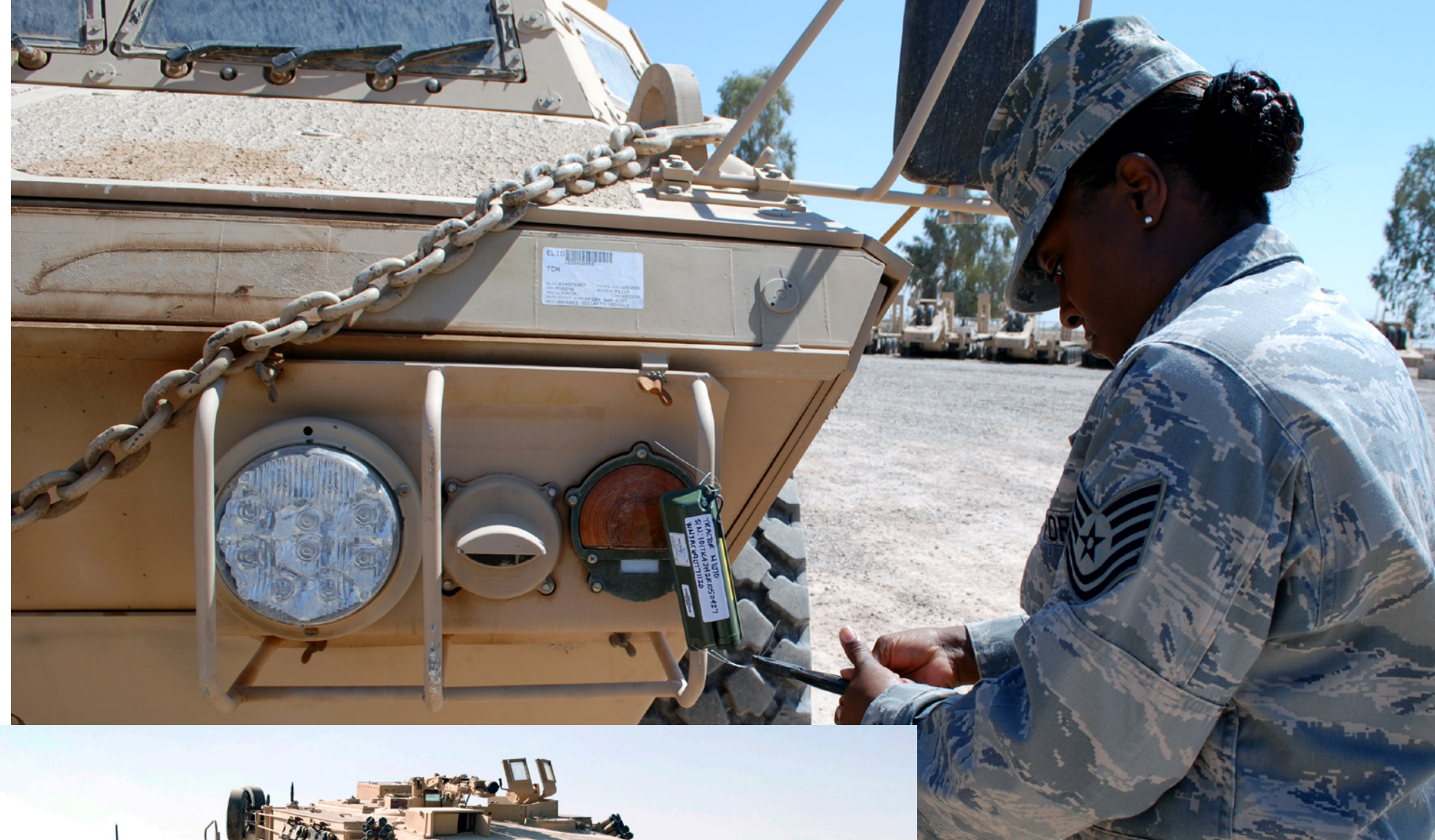
Air Force Tech. Sgt. Tamekah S. Burrell, a container management noncommissioned officer at one of the Redistribution Property Assistance Teams at Joint Base Balad, Iraq, attaches a radio frequency identification tag to a vehicle, enabling property accountability as materiel moves out of Iraq. The RPATs are overseen by AMC's 402nd Army Field Support Brigade. Photo by Summer Barkley, 402d Army Field Support Brigade.
