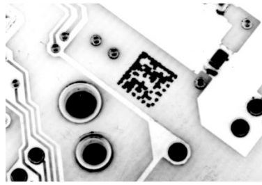
Figure 22 – Data Matrix Code Directly Marked on PCB Surface by Using Laser Etching Technology
