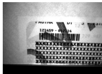
Figure 16 – Overprinted Barcode Readable by Matrix 300N also Through the Envelope Window Film
