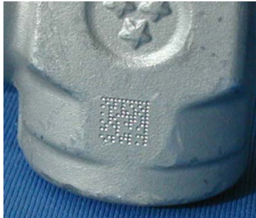
Figure 18 – Dot Matrix Code Directly Marked on Metal Surface by Using Dot Peening Technology
