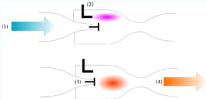
Pulse jet schematic. First part of the cycle: air intake (1), mixed with fuel (2). Second part: the valve (3) is closed and the ignited fuel-air mix (4) propels the craft.
