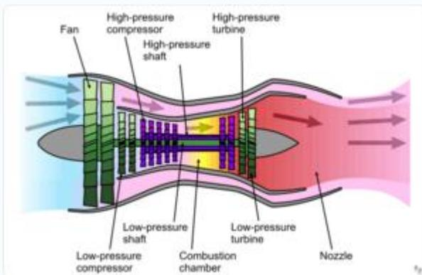
Schematic diagram illustrating a 2-spool, low-bypass turbofan engine with a mixed exhaust. The low-pressure spool is coloured green and the high-pressure one purple. The fan is driven by the low-pressure spool
