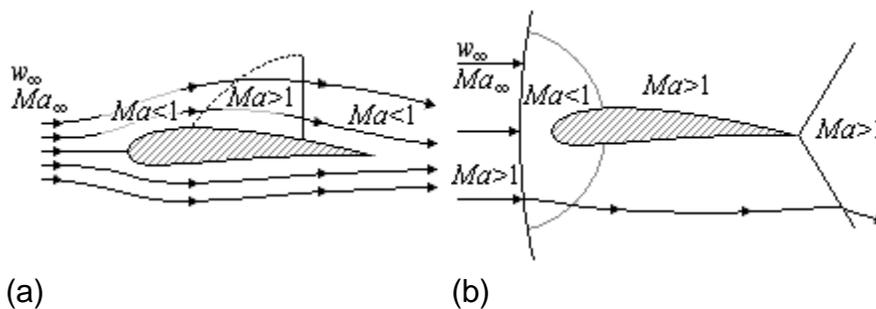
**Fig. 1.** Mach number in transsonic airflow around an airfoil;  $Ma < 1$  (a) and  $Ma > 1$  (b).
