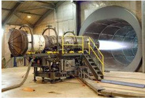
A Pratt and Whitney [turbofan](#) engine for the [F-15 Eagle](#) is tested at Robins Air Force Base, Georgia, USA. The tunnel behind the engine muffles noise and allows exhaust to escape. The mesh cover at the front of the engine (left of photo) prevents debris—or people—from being pulled into the engine by the huge volume of air rushing into the inlet.
