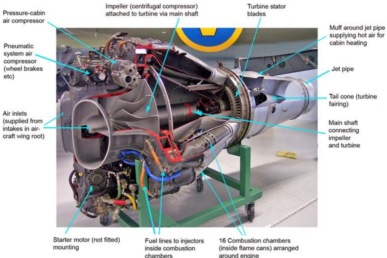
A picture of an early centrifugal engine (the [DH Goblin II](#)) sectioned to show its internal components
