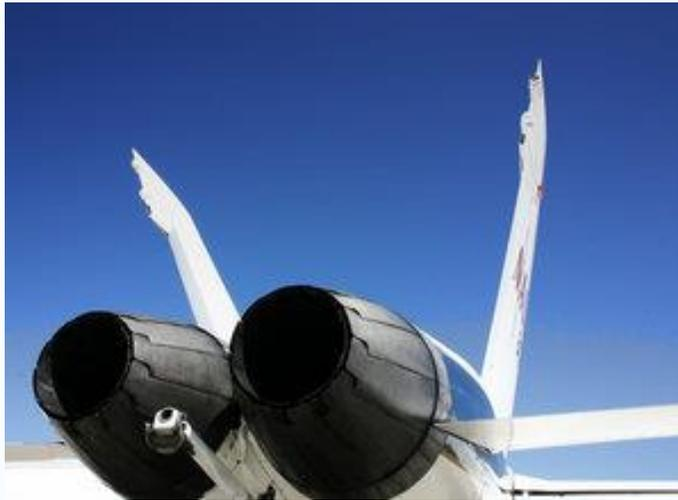
An afterburner injects fuel into the path of the hot exhaust gases to provide extra thrust.
