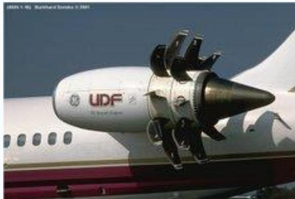
[General Electric GE-36](#) UDF Unducted Fan engine on a [McDonnell Douglas MD-81](#) testbed
