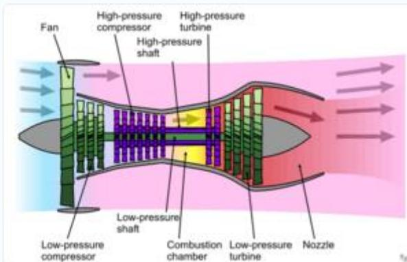
Schematic diagram illustrating a 2-spool, high-bypass turbofan engine with an unmixed exhaust. The low-pressure spool is coloured green and the high-pressure one purple. The fan is driven by the low-pressure spool.
