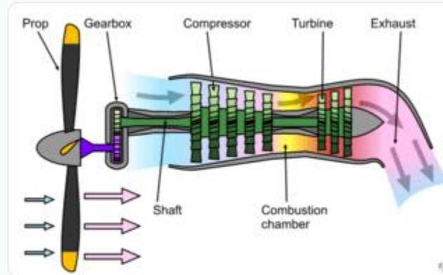
A schematic diagram showing the operation of a turboprop engine.
