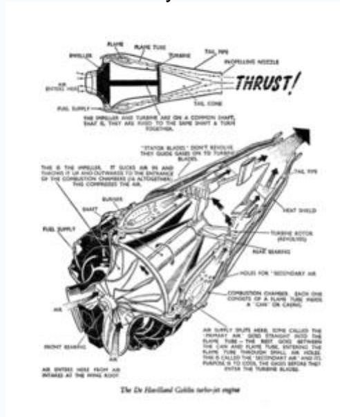
A cutaway diagram of the internal workings of the *de Havilland Goblin*, as fitted to the [Vampire](#).
