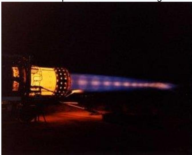
Pratt & Whitney J58 engine on testbed with full afterburner
