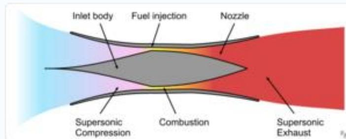
Diagram illustrating the principle of scramjet operation
