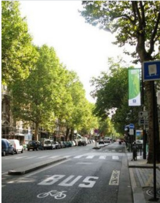
BICYCLE-BUS LANE: Located in Paris. The sign on the curb specifies hours when deliveries are allowed as long as the trucks pull halfway onto the sidewalk.
