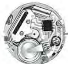
ESA/ETA 12 1/2''' 940 "FLATLINE QUARTZ" H 3.70, center second, instantaneous changing of date indication, with cor- rector and stop-second.
