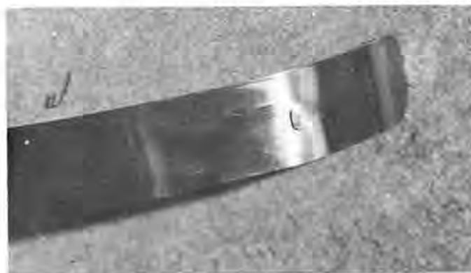
Figure 4. 3/4 Round or "D" shaped mainspring hook.
