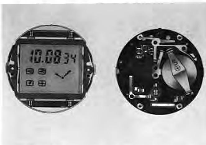
A new solid-state module with multiplexed display featuring six digits, 4 flags (function symbols) and 2 electronic hands. The digital readout has the following functions: time of day (12 or 24-hour cycle), minutes and seconds or date and day, 24-hour countdown timer, alarm with modulated signal, second time zone chronograph to the 1/100th second and intermediate times, night-light.
