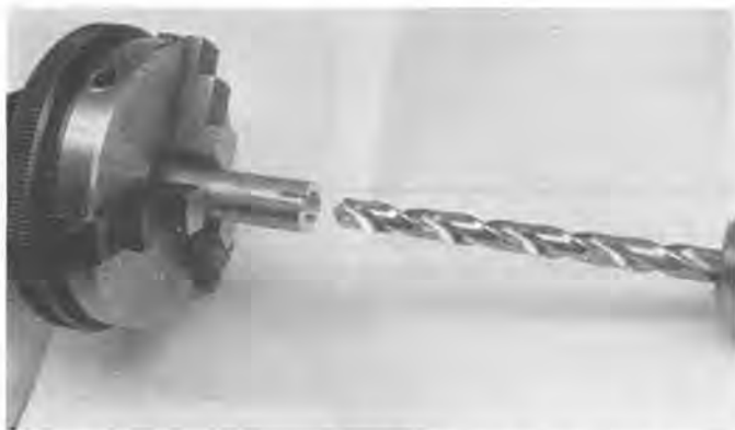
2) Drill your brass a bit under size, then broach to fit the hour pipe.
