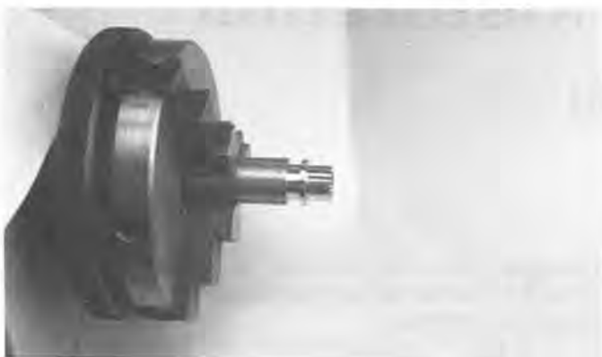
3) Turn the bush to fit hand with a suitable shoulder and cut off.
